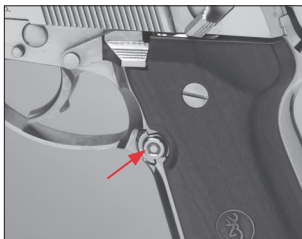
Press the magazine release button.
