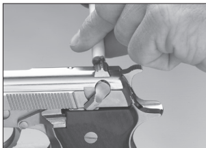
Gently tap the rear sight to adjust windage.
